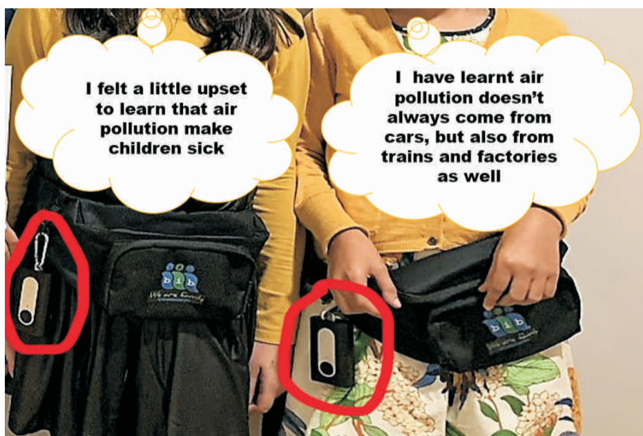
Figure 2: School kids with mobile sensors (Atmotube Pro), mobile phones in the bum bag record GPS position
